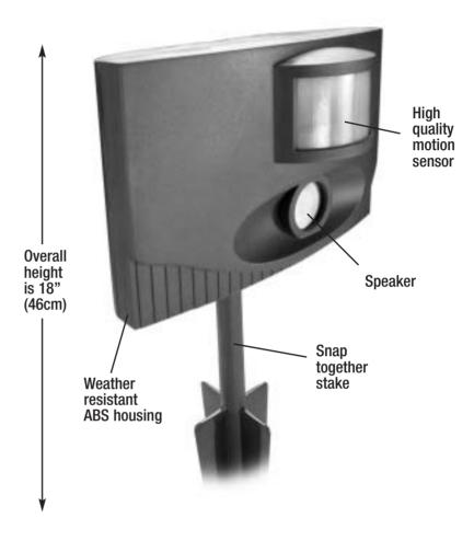
This unit can operate for up to nine months on one standard 9 volt battery. [Battery life estimate is based upon 4900 activations spread over 245 days at an average of 20 per day.]
